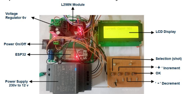
Figure 7. Electronics implementation of the prototype system.
